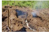
Earth Kiln – 10% Extremely inefficient Done on site where trees are cut
