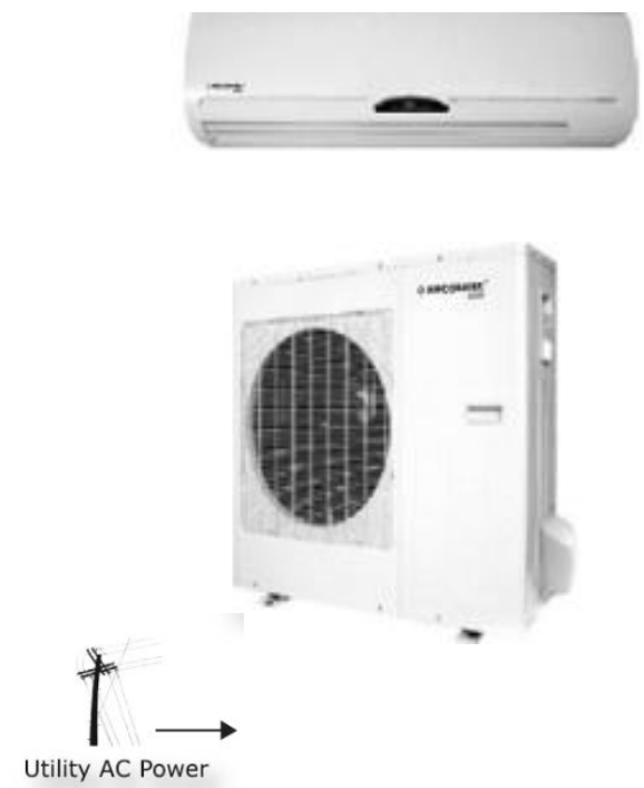
Conventional AC driven grid connected air-conditioning system
